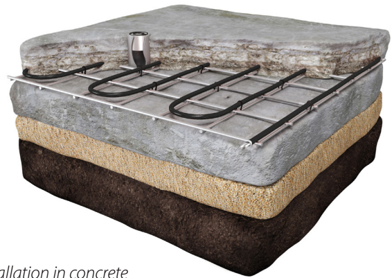
Installation in concrete
